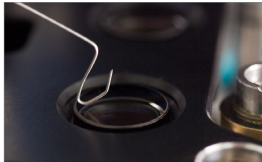
When the micro clapper of the computer controlled glue leveling machine brings eZoom's lens in the zoom body into position...
